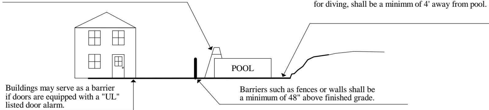
Latch may be located on the inside or outside of the gate if is 54" minimum above finished grade
